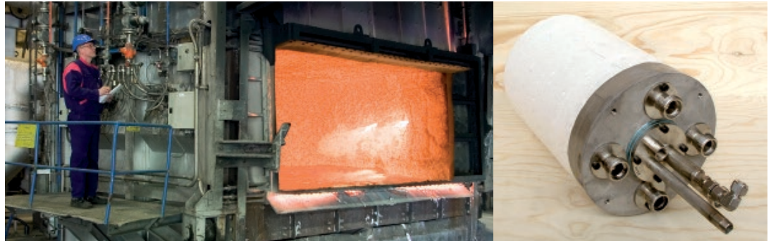
Low-temperature oxyfuel burner in the melt shop at SAPA Heat Transfer, Sweden.
